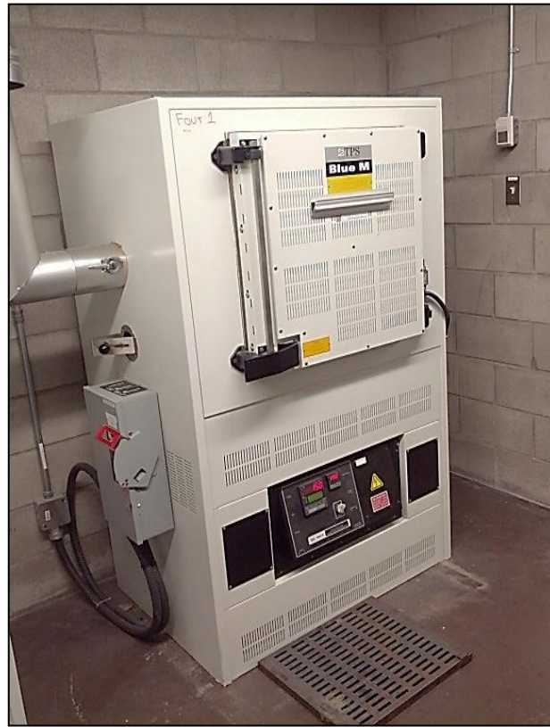
Figure 3.5 Blue M furnace used for heat treatment.
