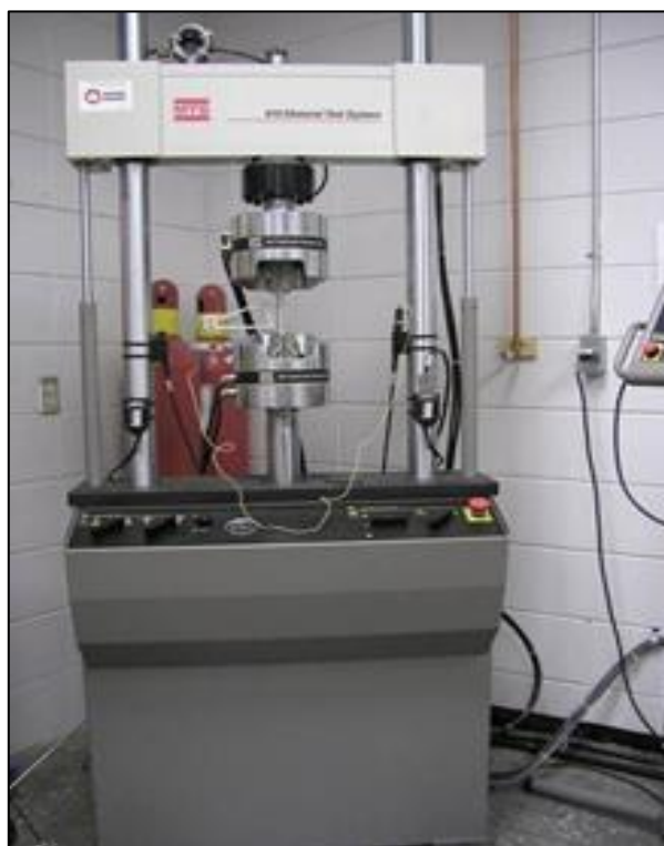
Figure 3.7 MTS Mechanical Testing machine used for room temperature testing.
