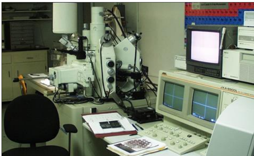
Figure 3.15 JEOL JXA-8900L WD/ED combined microanalyzer (EPMA) system used in the current study.
