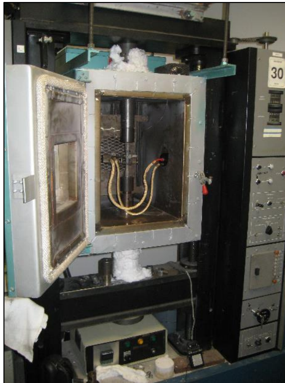
Figure 3.6 Instron Universal mechanical testing machine with chamber for high temperature testing.
