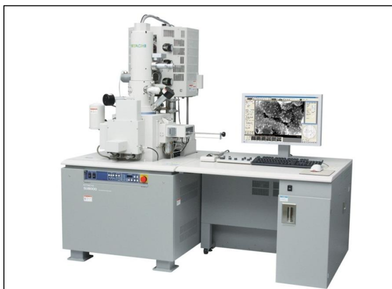
Figure 3.14 Hitachi-SU-8000 field emission scanning electron microscope used in the current study.
