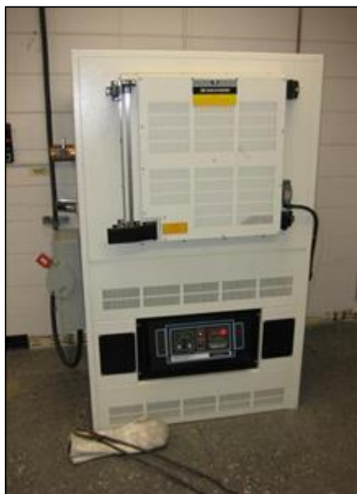
Figure 3.5 Lindberg Blue M electric furnace.
