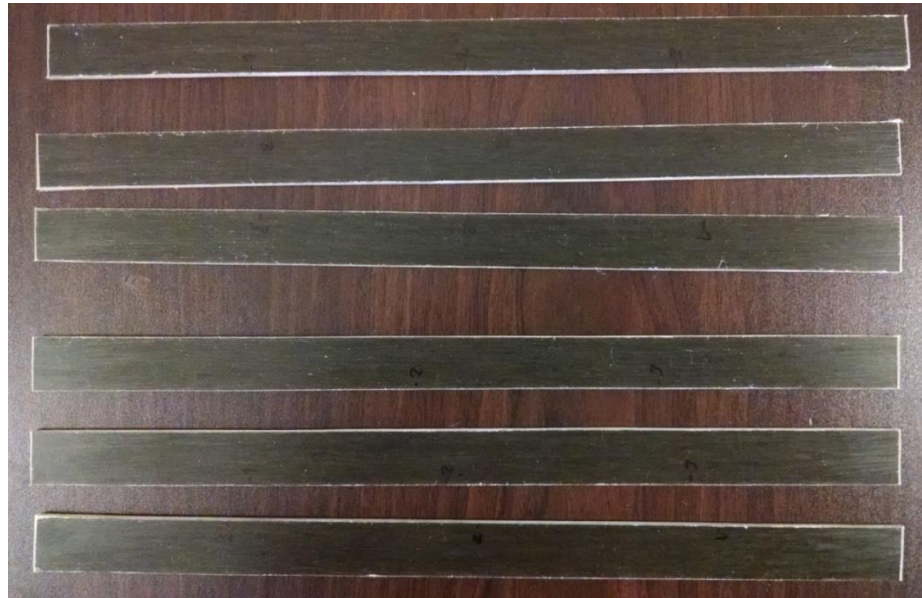
Figure 3-28. Tensile test coupons of the flax/paper composite (15 mm × 250 mm).
