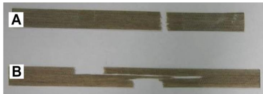
Figure 2-4. Results of tensile test on composite samples made of a layer of flax with (a) and without (b) paper [71]
