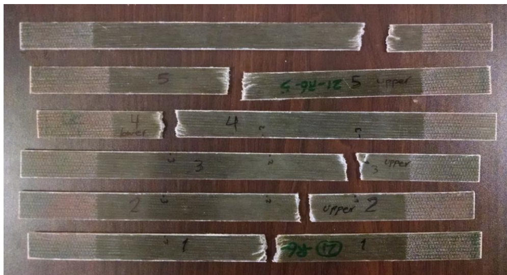
Figure 3-30. Typical tensile-test coupons after test.
