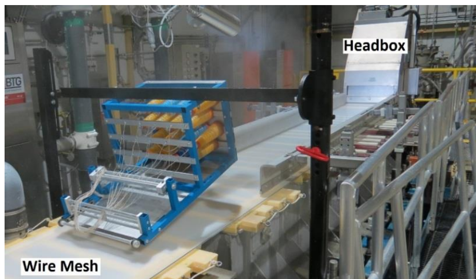
Figure 3-15. Installed feeding frame on the paper machine forming table.
