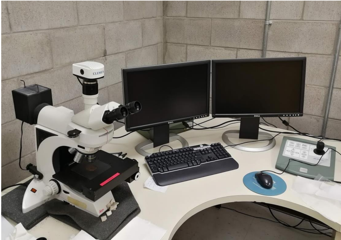
Figure 3-4 Optical microscope-Clemex Vision PE 4.0 image analyzer system
