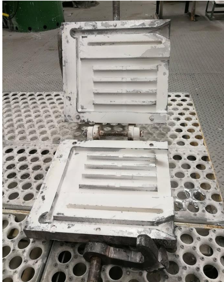
Figure 3-2 Waffle-Shaped Permanent Mold
