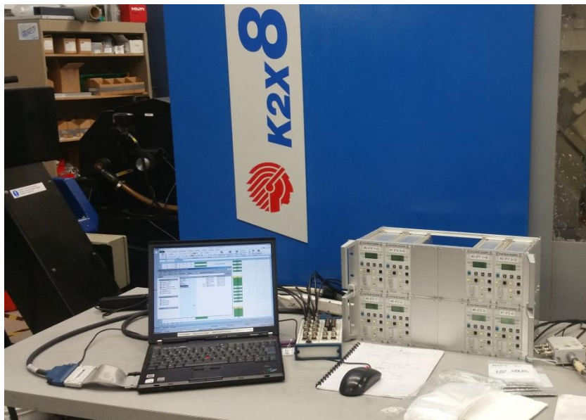
Figure 3-8 Hardware Configuration and Analogue-to-Digital Unit
