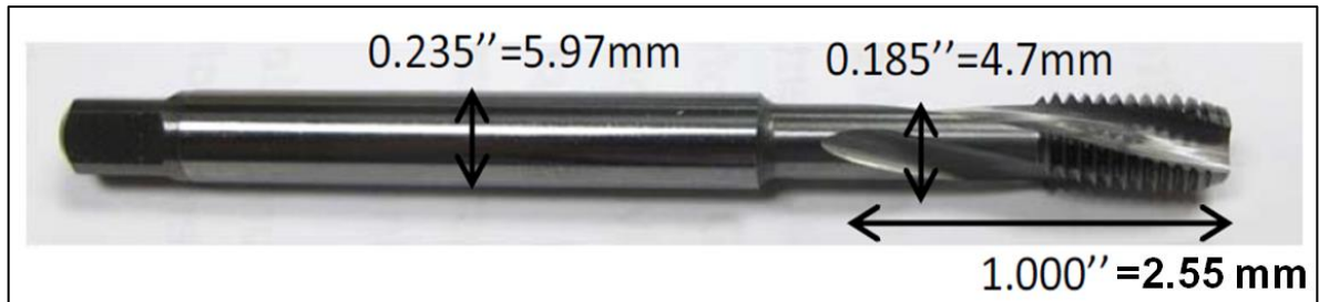
Figure 4-16 Shape and dimensions of the tapping tool used in the present study
