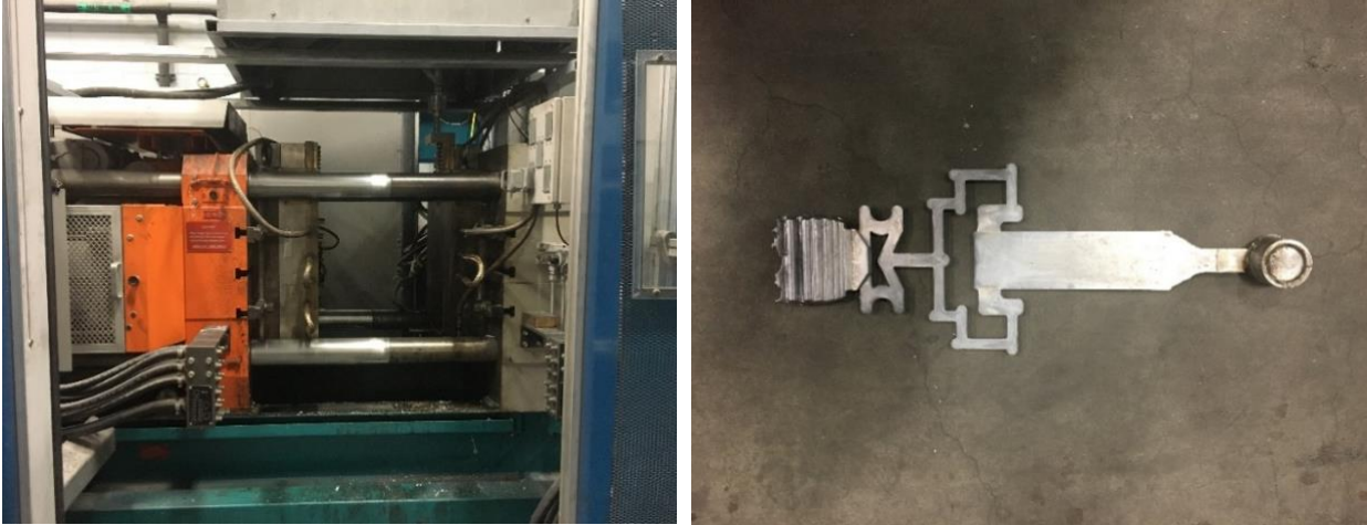
Figure 3-3: High pressure vacuum die casting machine and produced cast plates of a sample
