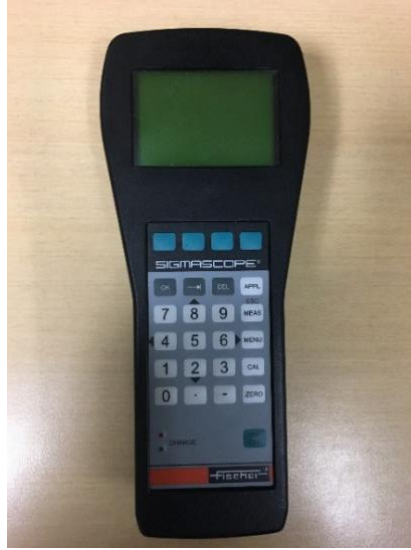
Figure 3-9: Portable Fisher Sigmacope Electrical Conductivity Measurement System
