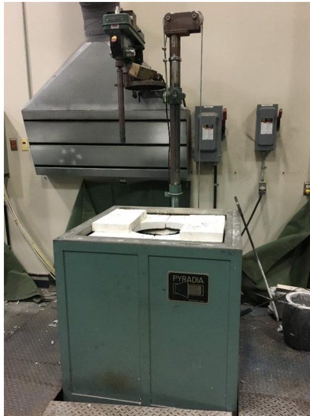
Figure 3-1: Electrical resistance furnace that used to produce the experimental alloys
