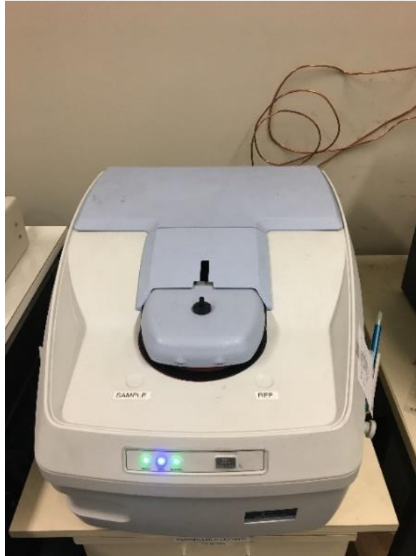
Figure 3-13: Differential scanning calorimetry system (DSC 8000) used in thermal analysis.
