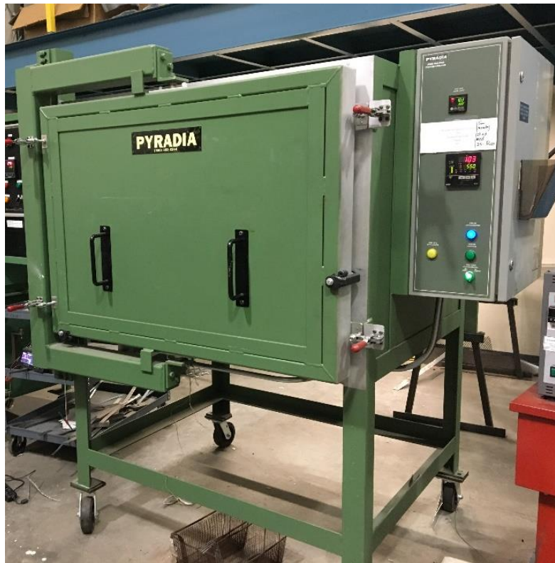
Figure 3-4: Electrical resistance furnace that was used for the heat treatments
