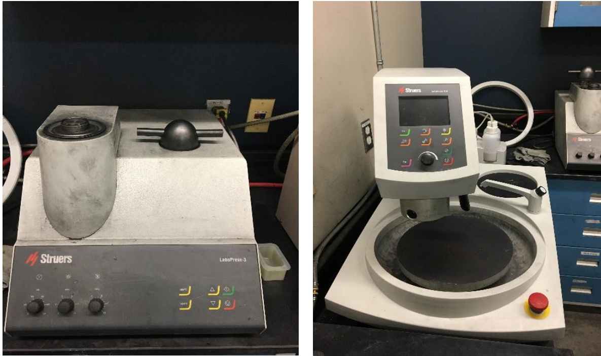
Figure 3-5: Mounting and polishing machines that used for the metallographic sample preparation
