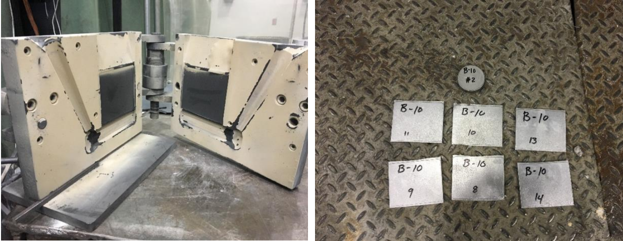
Figure 3-2: Permanent mold that was used to produce the experimental alloys and cast plates of the Base10 alloy
