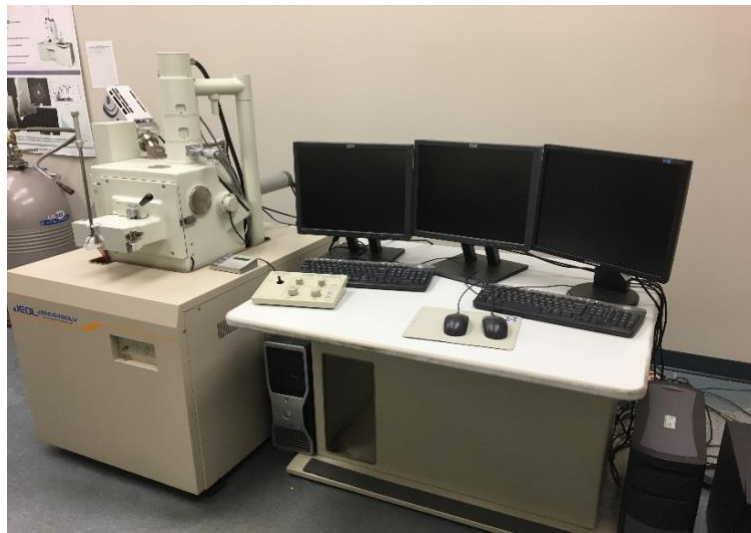
Figure 3-7: Scanning electron microscope used for microstructure observations
