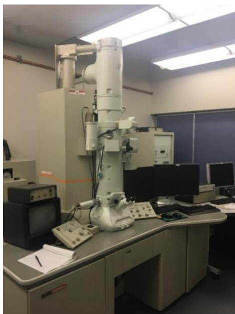
Figure 3-8: TEM, JEM-2100 transmission electron microscope.
