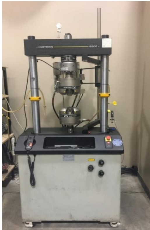
Figure 3-12: Instron-8801 tensile testing machine.
