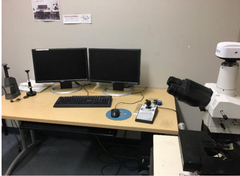
Figure 3-6: Nikon Eclipse ME600 Optical Microscope
