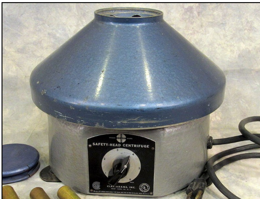
Figure VI-3: Laboratory setup used for centrifugal treatment.
