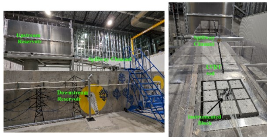
Fig. 1. Laboratory spillway model with 15X15X30 cm blocks at the end of spillway channel.
