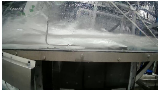
Fig. 13. Development of hydraulic jump at protruded surface for configuration 3.
