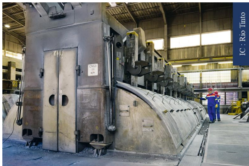
Figure 1-3 : Industrial aluminium reduction cell in operation at LRF, Saint-Jean-de-Maurienne, France
