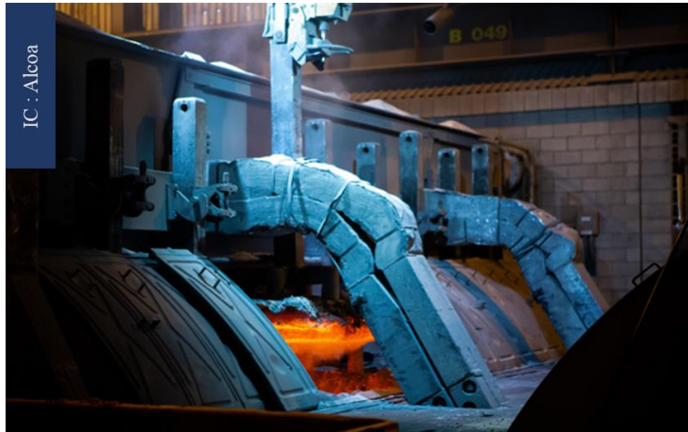
Figure 2-15 : Anode change operation in a prebake reduction cell
