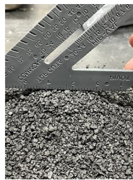
(b) Measurement of the top diameter
