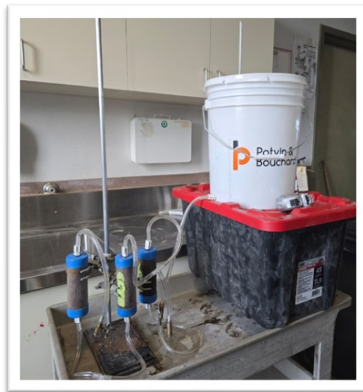
Figure 14: Experimental setup for leaching dissolved organic carbon (DOC).
