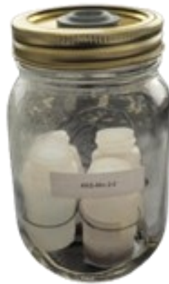
Figure 10: Sealed incubation chamber for measuring soil microbial respiration.
