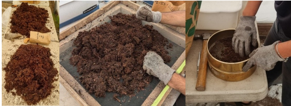
Figure 5: The separation (left panel), 5-mm sieving (middle panel), and 2-mm sieving (right panel) of the soil samples.
