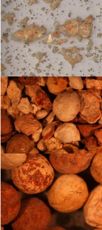
Figure 36: Particles of bauxite (from the top to the bottom: 45 \mu m, 1mm, 4mm)
