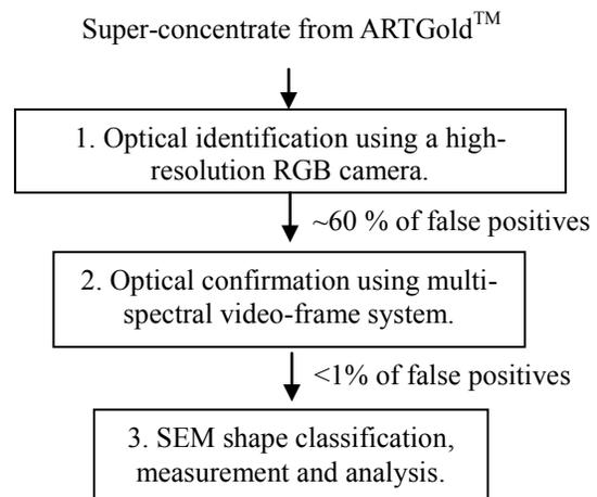
**Figure 3.** Flow chart summarizing the identification process from the super-concentrated heavy minerals to SEM classification and measurement.
