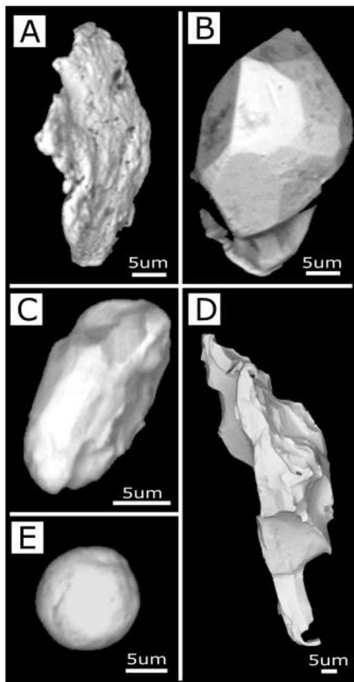
**Figure 5.** Pristine gold grains classification. **a** Remobilized, **b** Crystalline, **c** Mutual, **d** Intergranular and **e** Spherule.
