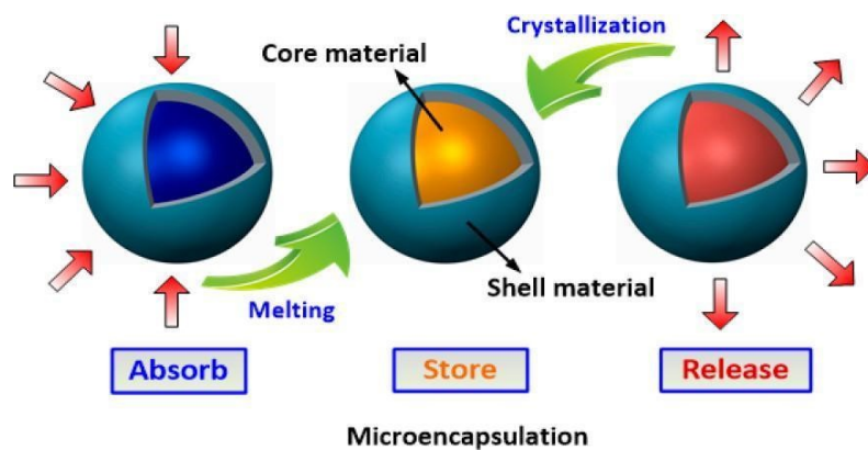
Figure 1-17. Schematic showing the structure of PCM microcapsules and PCM release [207].
