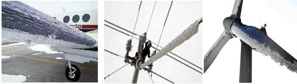
Figure 1-1. Ice build-up on an aircraft wing (left), a high-voltage electrical line (middle), and wind turbine blades (right) [6].
