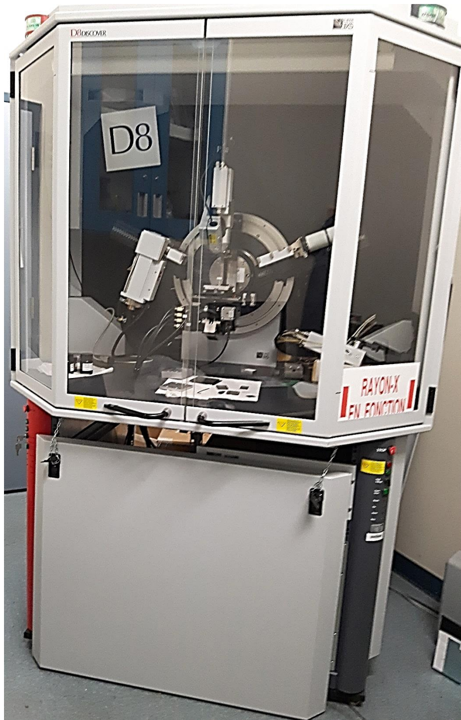
Figure 3-8. Digital image of X-ray diffractometer, Bruker D8 Discover system, CURAL, UQAC. © Henry Agbe, 2021
