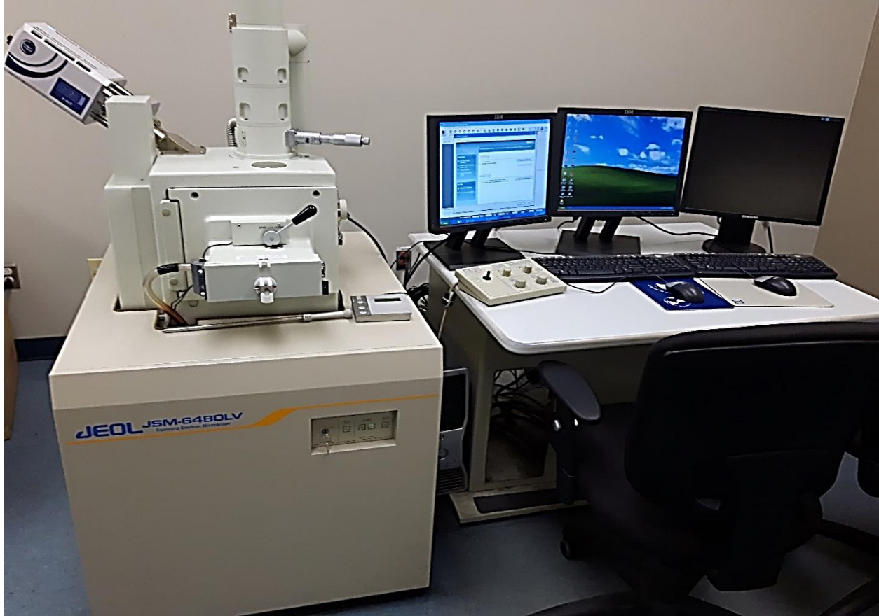
Figure 3-5. Digital image of scanning electron microscope (model SEM JEOL JSM 6480LV), CURAL, UQAC. © Henry Agbe, 2021
