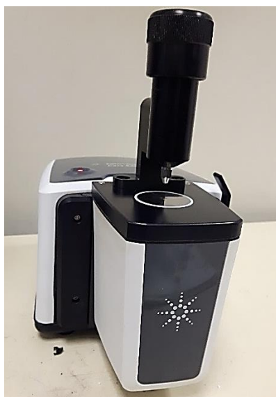
Figure 3-6. Digital image of Fourier transform infrared spectroscopy instrument (ATR-FTIR) Cary 630 Agilent Technologies, CURAL, UQAC. © Henry Agbe, 2021
