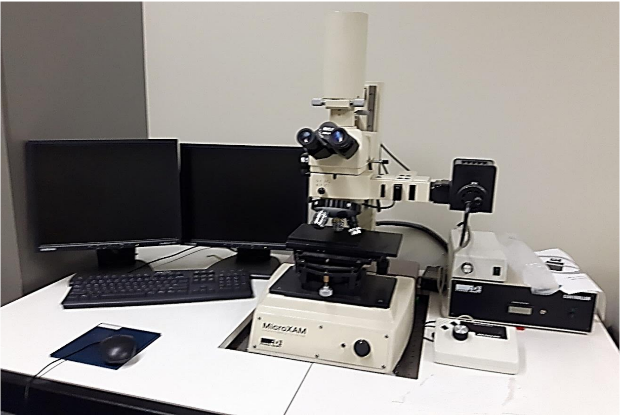
Figure 3-9. Digital image of the optical profilometer, CURAL, UQAC. © Henry Agbe, 2021
