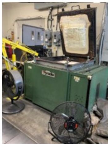
Figure 3.5. Electrical anode baking furnace at UQAC
