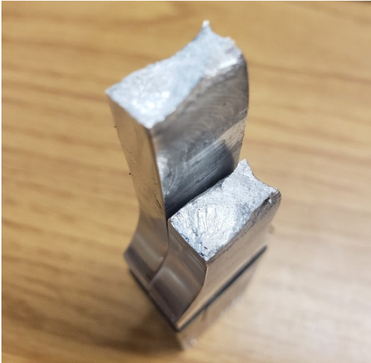
Figure C.17.FL8- Rupture dans ZM
