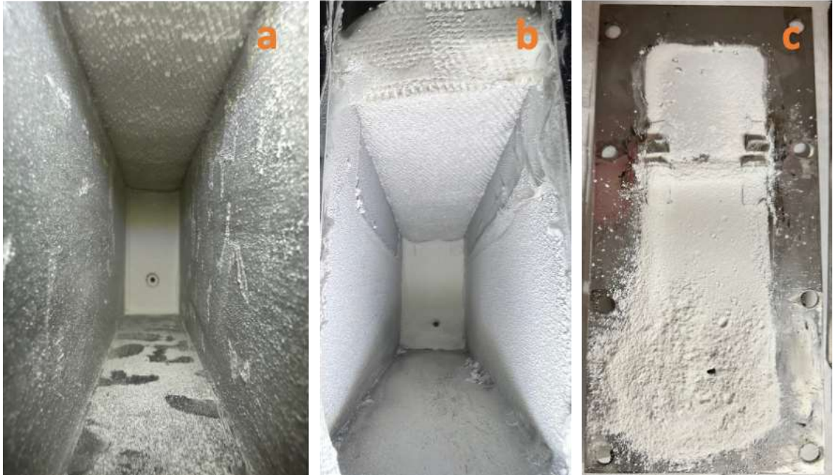
Figure A 3. Images of the reactor system at (a) 5 min, (b) 15 min, and (c) deposited lime on the bottom plate after reaction
