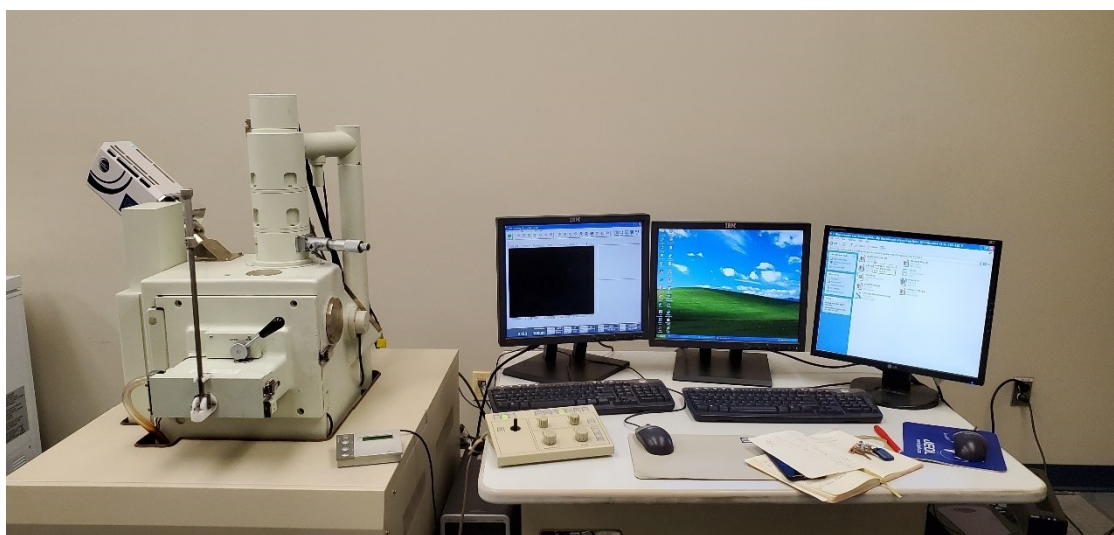
Figure 3.4 Scanning Electron Microscope SEM Jeol (model JSM 6480LV) instrument (at the laboratory of CURAL, UQAC).
