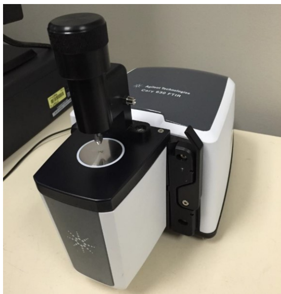
Figure 3.3 Attenuated Total Reflectance-Fourier Transform Infrared Spectroscopy (ATR-FTIR) Cary 630 Agilent Technologies instrument (at the laboratory of CURAL, UQAC).
