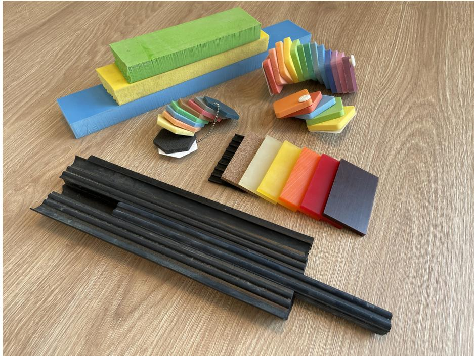
Figure 2.11: Various types of viscoelastic interlayers commonly used in wooden buildings.
