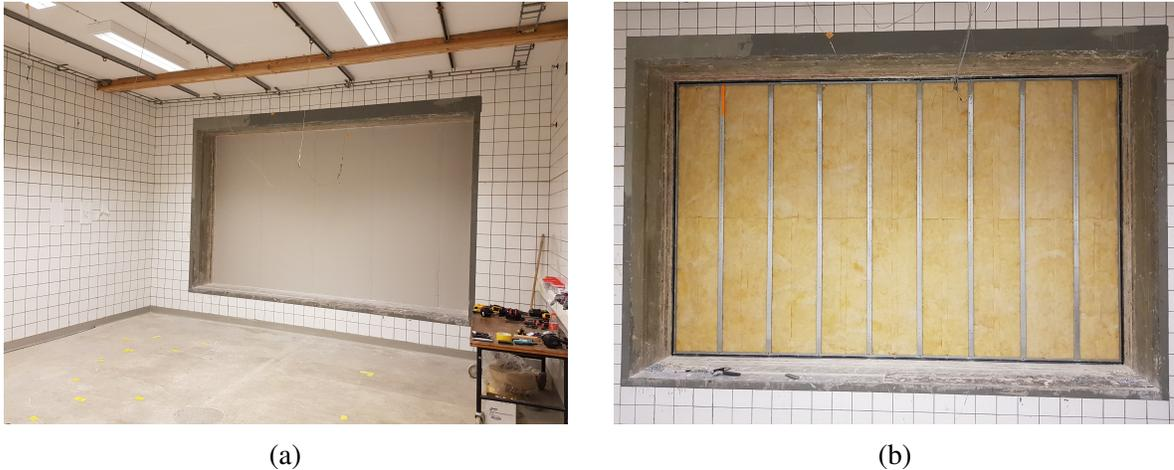
Figure 3.2: Pictures from the measurements of the separating reference wall: (a) The finished mounted wall; (b) The inside of the wall with a sound reduction index of  $R_w$ : 54 dB.
