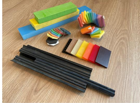
Figure 5.2: Viscoelastic interlayers from different manufacturers in a building (left) and as samples (right).
