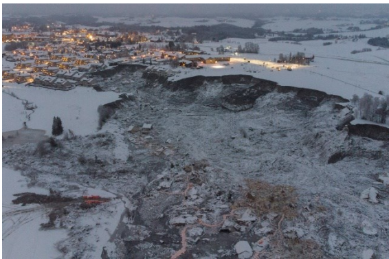
Figure 3. Retrogressive landslide in the sensitive clays of Gjerdrum in Eastern Norway on December 30, 2020 (Photo: Anders Martinsen)
