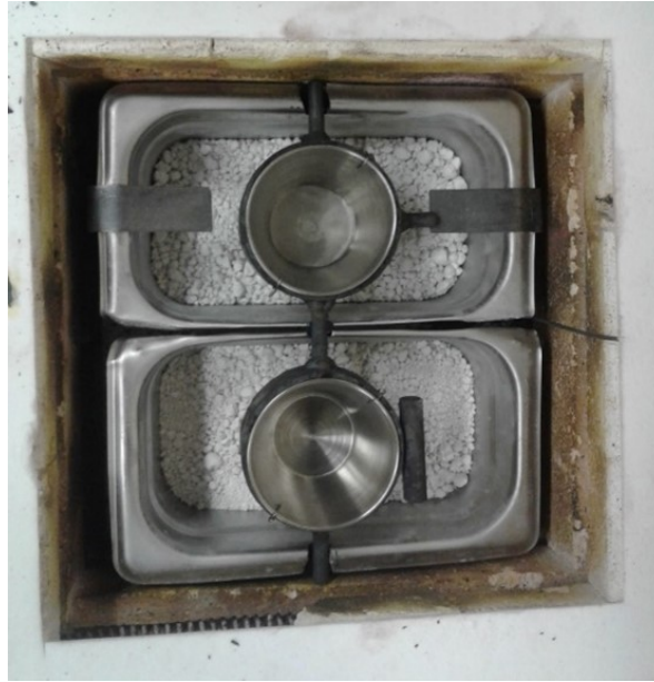
Figure 2.7 : Experimental setup for the tests on the sintering of alumina
