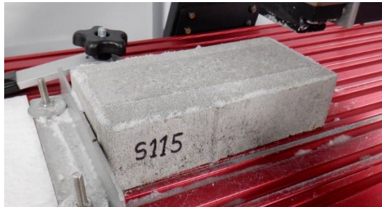
Figure 13: Removed snow condition with standard concrete sample (RWYCC 4)
