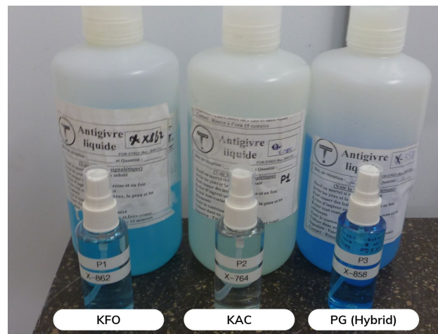
Figure 16: Runway De-Icing-Icing Products (KFO, KAC, and PG Hybrid)
