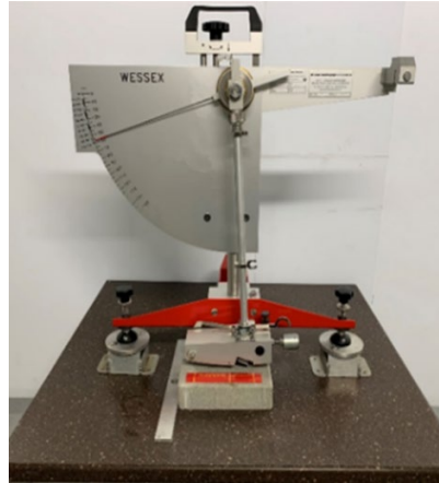
Figure 6: British Pendulum Tester at the Anti-Icing Materials International Laboratory.
