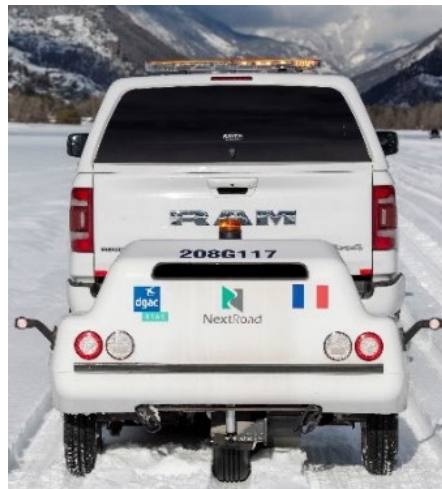
Figure 8: Automatic Slip Measurement Instrument (IMAG) [74] © Richard METZGER / DGAC — STAC.
