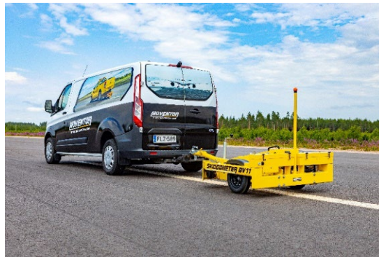
Figure 9: Skiddometer BV-11 [79]. © Moventor Oy, 2024
