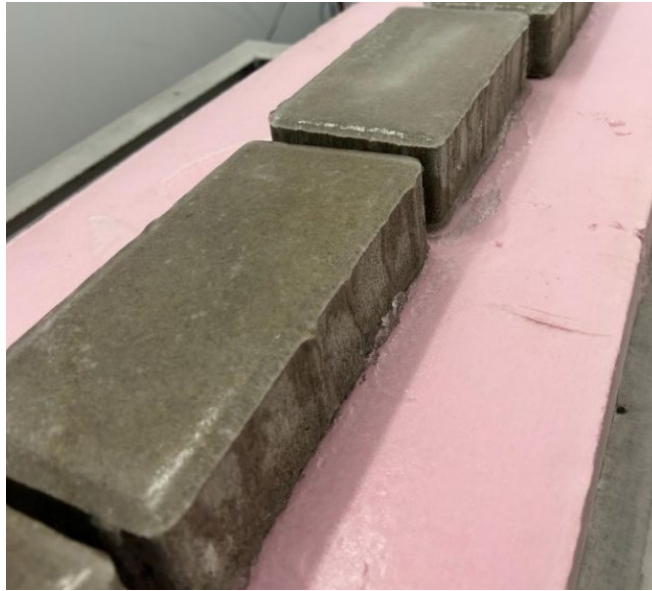
Figure 18: Concrete samples after icing in the cold room.
