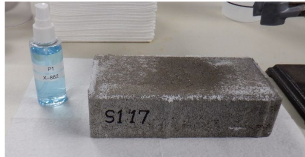
Figure 25: De-icing test with removed snow condition and KFO
