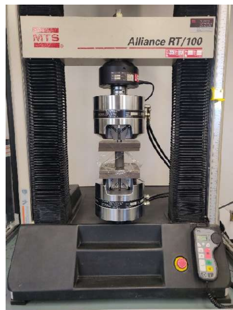
Figure 2. A sample placed inside the uniaxial compression testing machine
