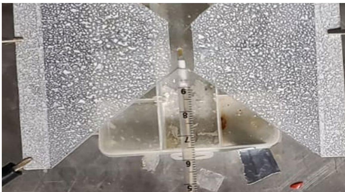
Figure 60 : EO probe centered on an artificial dry band.
