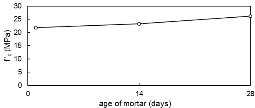
Fig. 1.2 – Effect of the age of the geopolymer mortar R60-40 on the average compressive strength, cure at 60°C during 24 h
