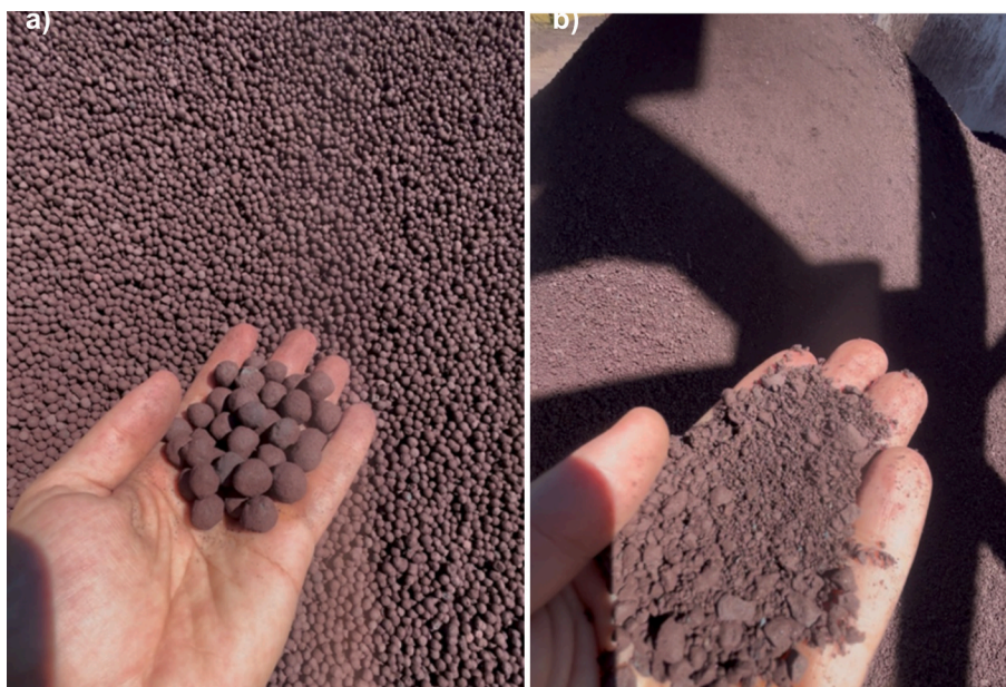
Fig. 8. (a) Screened iron ore fired pellets (final product). b) Rejected material (<5.0 mm).
