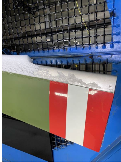
Figure 2.12. Fracture of the ice on rotor blade for hard mixed ice.
