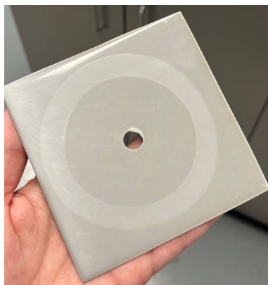
Figure 3.8. Surface of the coating after abrasion test, exhibiting minimal wear and no significant damage.
