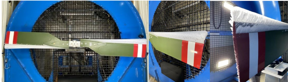
Figure 2.11. Hard mixed ice at -12°C, a) Complete rotor. b) Single blade from the front. c) Single blade from behind.
