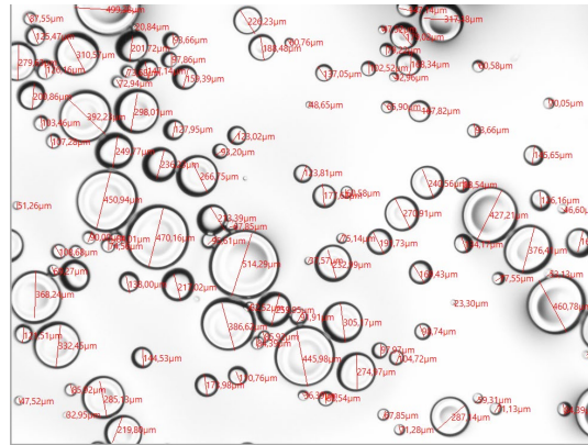
Figure 2.2. Measurement method used to determine the mean volume diameter (MVD) of droplets.
