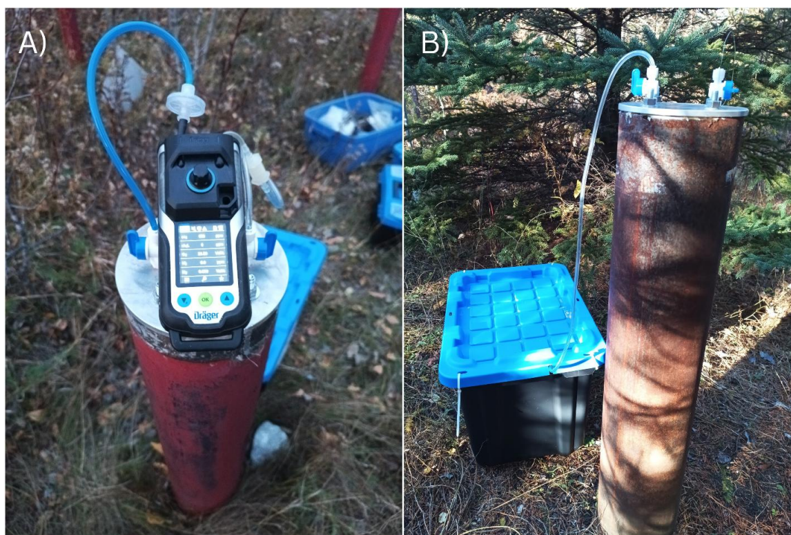
Fig. 4 A) Gas detector Draeger X-Am 8000 connected to the valves of the sealed wellhead cap. B) In situ free gas sampling setup from a dedicated wellhead during the measurement intervals (without the gas detector connected).
