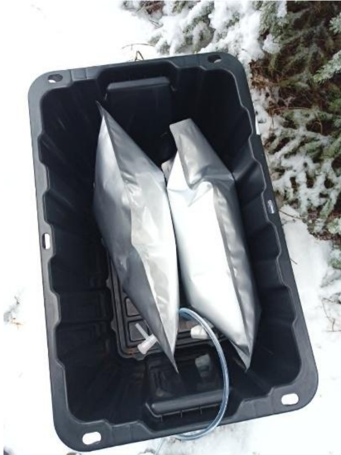
Fig. 10 Bin containing gas sampling bags from the FA-1 well. The volume of gas recovered (after correction for P and T) was approximately 12L.
