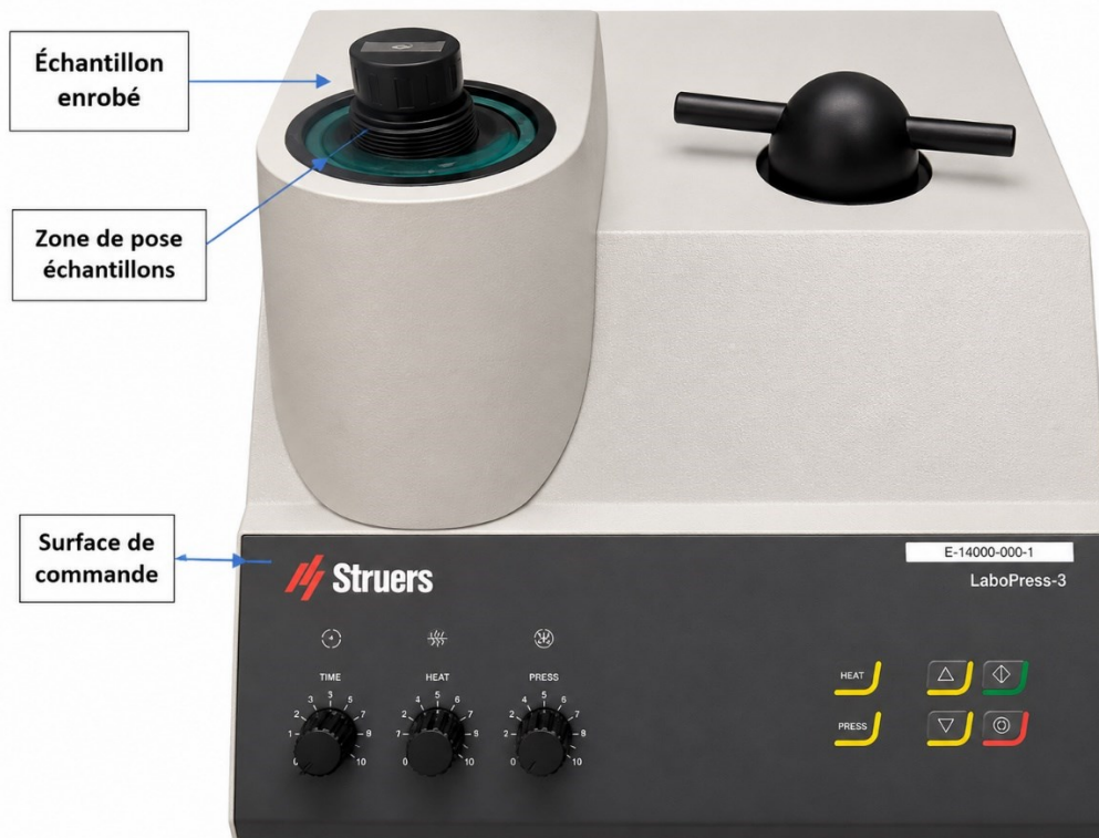
Figure 3-22: Machine d'enrobage Struer LaboPress-3
