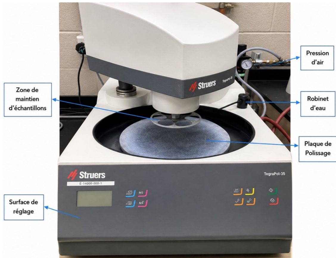
Figure 3-23: Machine de polissage
