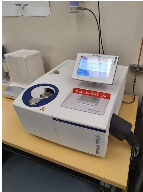
Figure 2.29 Machine d'analyse METTLER TOLEDO DSC3 StarSystem [72]
