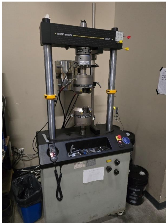
Figure 2.34 Presse de traction hydraulique Instron® 8801 [78]
