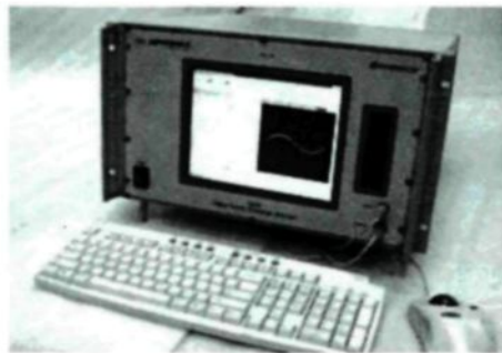
Figure 1.5. Partial Discharge Detector (DDX 7000).
