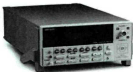
Figure 1.6. Model 6517A electrometer/high resistance meter.
