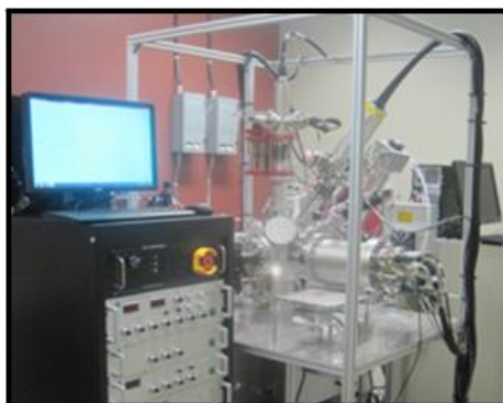
Fig.3.5. X-ray photoelectron spectroscopy (XPS) instruments, CIGELE laboratory.
