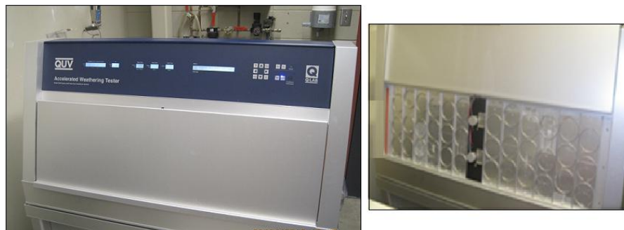
Fig.3.11. QUV accelerated weathering tester apparatus, CIGELE laboratory ( left ) and inside of sample chamber ( right ).
