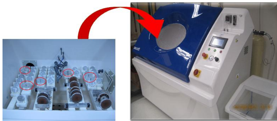
Fig.3.14. A programmable cyclic corrosion test chamber ( Ascott ), NRC-ATC.
