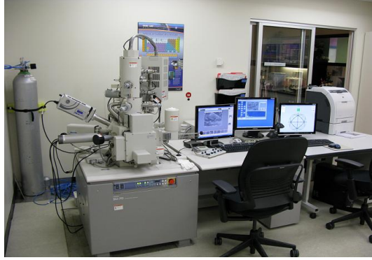
Fig.3.3. Image of scanning electron microscope (SEM) used in the present study (ATC lab).
