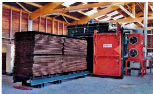
Figure 2.1 Wood Heat Treatment Furnace [7]
