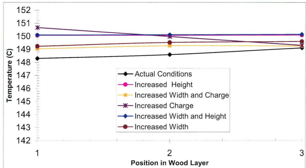
Figure 6.44 Comparison of Predicted Wood Temperature in the Bottom Wood Layer after Six Hours of Operation.
