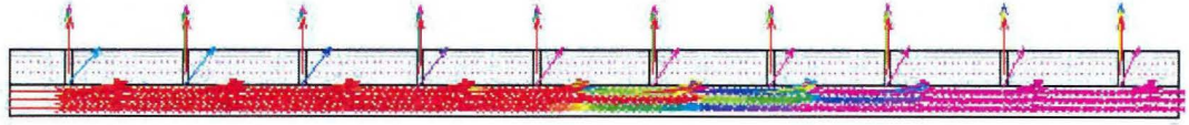
Figure 3.9 Velocity Distribution of the Gas in the Channel for Inlets with Nozzle (Top View)
