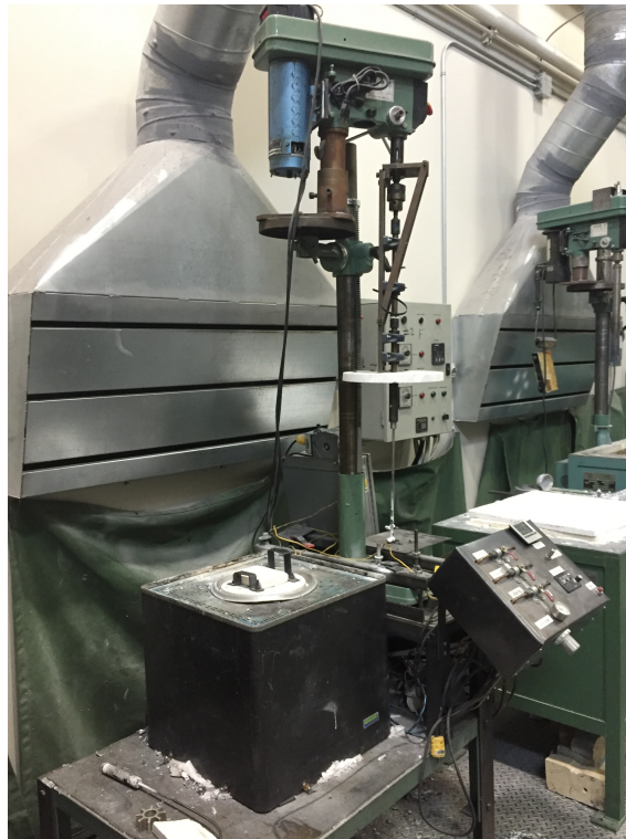
Fig. 3. 1. The electric resistance furnace used for composites preparation with a controllable stirring facility.
