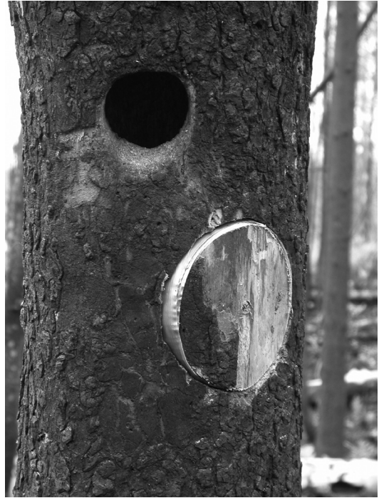
Fig. 2. Opening closed using the wooden disc produced by the hole saw. Note that wrapping several layers of duct tape around the wooden disc ensures a tight fit.
