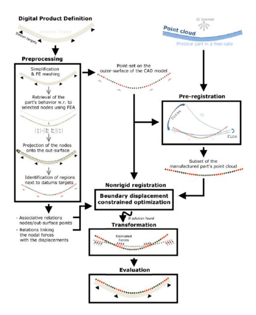
Figure 2-6: Schematic flowchart of proposed *virtual fixture* method in (Abenhaim, Desrochers et al. 2015).
