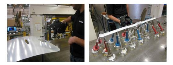
Figure 4-2: Surface data acquisition by a handy scanner.
