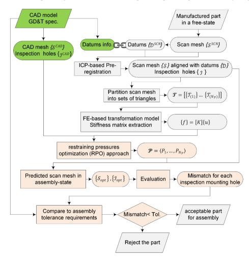
Figure 6-6: Flowchart algorithm of proposed VMASI method.
