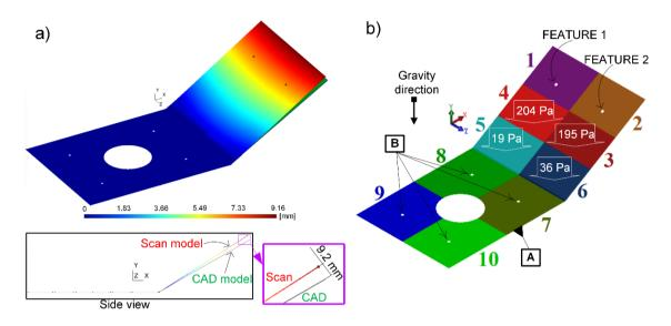
Figure 6-12: a) Displacement distribution [mm] of slightly deviated scan mesh simulating a plastic defect; b) The partitioned scan model and predicted assembly pressure.
