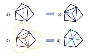
Figure 4-6: a) The purple point presents a GNIF sample point to be inserted b) the sample point is inserted into the mesh by incremental Delaunay triangulation c) Testing the empty sphere criterion d) swap diagonal operator.
