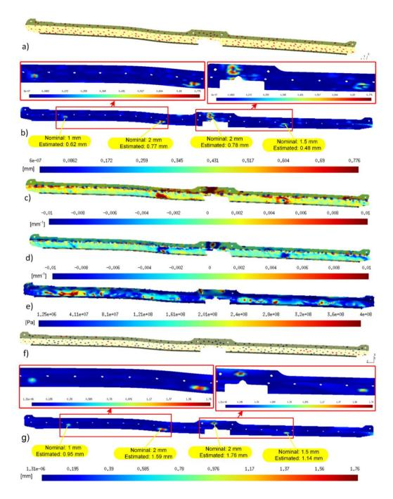
Figure 4-30: Part B with small (local) defects and torsion a) and f) initial and filtered sample points c) and d) distribution of the difference in principle curvatures [mm<sup>-1</sup>] e) distribution of von Mises stress [Pa] after the second FENR. b) and g) comparison between estimated and nominal size of defects [mm] based on initial and filtered sample points.
