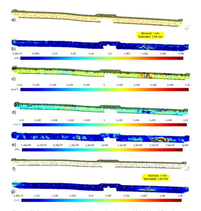
Figure 4-32: Part B with a big (global) defect and torsion a) and f) initial and filtered sample points c) and d) distribution of the difference in principle curvatures [mm<sup>-1</sup>] e) distribution of von Mises stress [Pa] after the second FENR. b) and g) comparison between estimated and nominal size of defects [mm] based on initial and filtered sample points.
