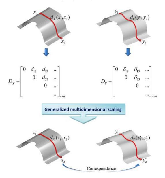
Figure A-3: Determining the correspondence between sample points (*number of sample points = n*) on the CAD and scan models ( $D_x$  and  $D_y$  represent symmetric matrices of pairwise geodesic distances, calculated by *fast marching algorithm*) (Radvar-Esfahlan 2010).
