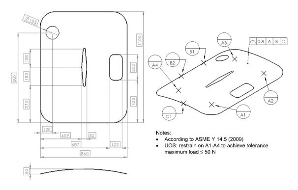
Figure 5-13: CAD model along with GD&T specification for part A (dimensions are in mm).
