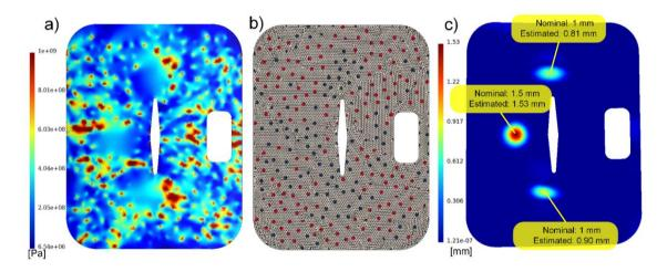
Figure 4-19: Part A with small (local) defects and torsion a) distribution of von Mises
