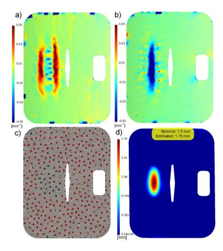
Figure 4-24: Part A with a big (global) defect and torsion a) distribution of the difference in maximum curvature  $(K_1)$  [mm<sup>-1</sup>] b) distribution of the difference in minimum curvature  $(K_1)$  [mm<sup>-1</sup>] c) sample points filtered using the curvature criterion (represented as blue spots) d) comparison between estimated and nominal size of defects [mm] when using GNIF sample points after filtering based on the curvature criterion.
