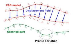
Figure 2-8: constructing deformed CAD model using displacement field without taking into consideration the presence of effects (Abenhaim, Tahan et al. 2011).
