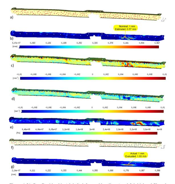
Figure 4-31: Part B with a big (global) defect and bending a) and f) initial and filtered sample points c) and d) distribution of the difference in principle curvatures [mm<sup>-1</sup>] e) distribution of von Mises stress [Pa] after the second FENR. b) and g) comparison between estimated and nominal size of defects [mm] based on initial and filtered sample points.
