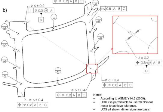
Figure 6-14: a) The manufactured part mounted on inspection fixtures where a real point cloud of scan mesh can be acquired, in our proposed method only 9 fixation features are kept as datums; b) GD&T specification for part B (dimensions are in mm).
