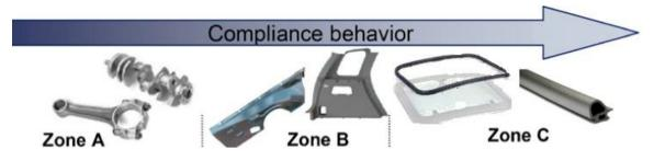
Figure 2-1: Classification of the compliant behavior of parts (Abenhaim, Desrochers et al. 2012).
