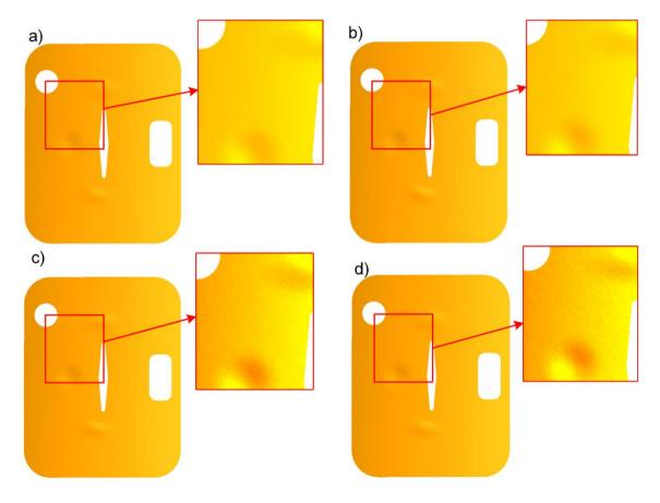
Figure 5-11: a) a noise-free scan mesh b), c), d) scan meshes with synthetic noise with Gaussian distribution with zero mean value and standard deviation equal to b) 0.01mm c) 0.02mm d) 0.03mm.
