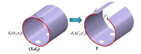
Figure 2-9: Distance preserving property of non-rigid part during an isometric deformation (Radvar-Esfahlan and Tahan 2014).
