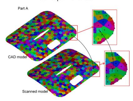
Figure 4-5: GNIF corresponding sample points (in black) are located in the center of colored zones on CAD and scanned models.
