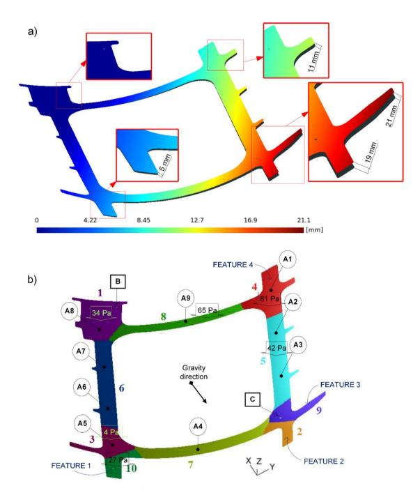
Figure 6-16: a) Displacement distribution [mm] of deviated scan mesh simulating an intermediate plastic defect; b) the partitioned scan model and predicted assembly pressure.
