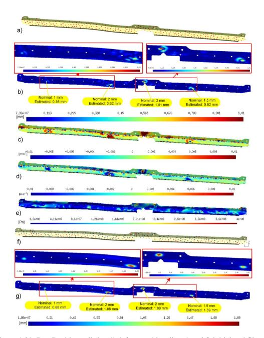
Figure 4-29: Part B with small (local) defects and bending a) and f) initial and filtered sample points c) and d) distribution of the difference in principle curvatures [mm<sup>-1</sup>] e) distribution of von Mises stress [Pa] after the second FENR. b) and g) comparison between estimated and nominal size of defects [mm] based on initial and filtered sample points.
