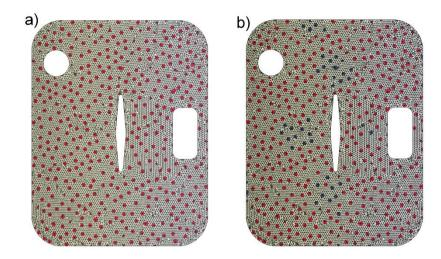
Figure 5-4: a) all GNIF sample points inserted into the CAD mesh based on classical Delaunay method (red spots) b) automatic sample point filtration based on curvature and von Mises stress criteria and criteria (blue spots).
