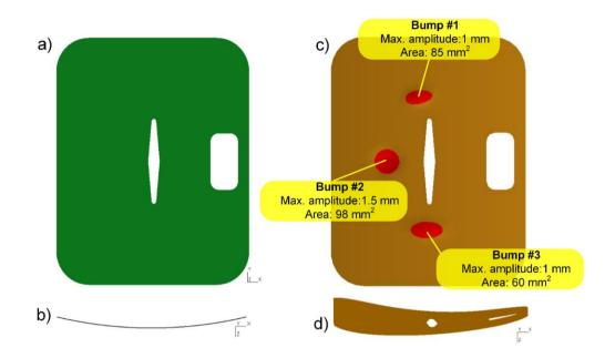
Figure 4-4: A non-rigid aluminum panel a) front view of the CAD model b) top view of the CAD model c) front view of the scanned part in a free-state d) top view of the scanned part in a free-state.
