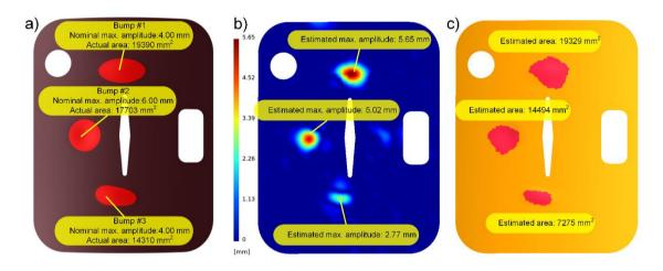
Figure 5-6: a) the scanned part with the nominal dimensions of defects b) estimated and nominal maximum amplitude  $(D_i^{max})$  of defects [mm] c) estimated and nominal area  $(A_i \text{ shown as red zones})$  of defects [mm<sup>2</sup>].
