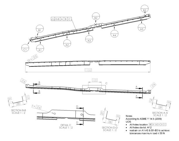
Figure 5-16: CAD model along with GD&T specification for part B (dimensions are in mm).
