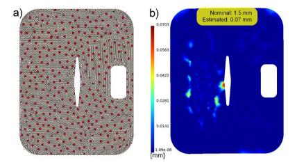
Figure 4-20: Part A with a big (global) defect and bending a) GNIF sample points on the CAD model represented as red spots b) comparison between estimated and nominal size of defects [mm] when using all GNIF sample points.
