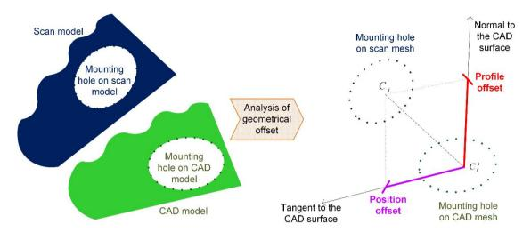
Figure 6-4: Analysis of geometrical offset based on GD&T specification.
