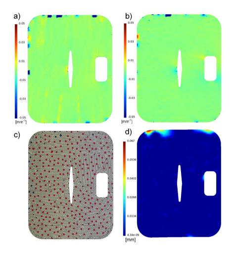
Figure 4-13: a) distribution of the difference in maximum curvature  $(K_1)$  [mm<sup>-1</sup>] b) distribution of the difference in minimum curvature  $(K_2)$  [mm<sup>-1</sup>] c) sample points filtered using the curvature criterion (represented as blue spots) d) comparison between deformed CAD and scanned models when using GNIF sample points after filtering based on the curvature criterion [mm].
