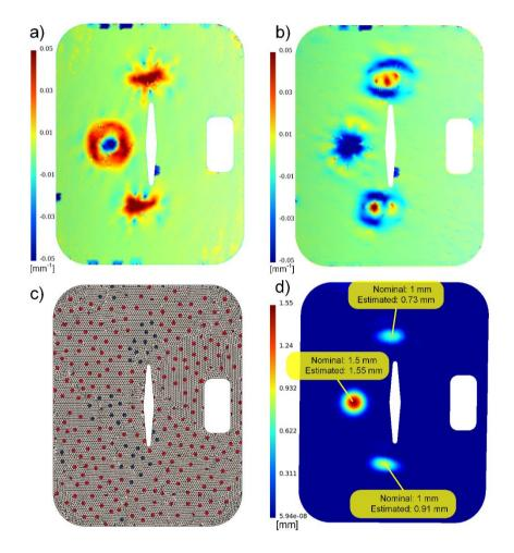
Figure 4-18: Part A with small (local) defects and torsion a) distribution of the difference in maximum curvature  $(K_1)$  [mm<sup>-1</sup>] b) distribution of the difference in minimum curvature  $(K_2)$  [mm<sup>-1</sup>] c) sample points filtered using the curvature criterion (represented as blue spots) d) comparison between estimated and nominal size of defects [mm] when using GNIF sample points after filtering based on the curvature criterion.
