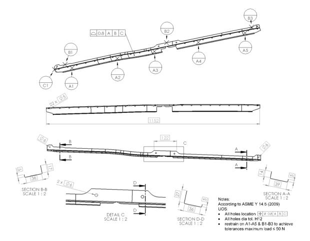
Figure 4-26: CAD model along with GD&T specification for part B (dimensions are in mm).
