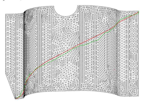
Figure A-2: Geodesic distance between two points on a triangulated mesh is better estimated with *Fast Marching Algorithm* (the red path) compared to *Dijkstra's shortest path algorithm* (the green path) (Radvar-Esfahlan 2010).
