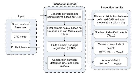
Figure 5-7: Flowchart of our automatic fixtureless CAI method.
