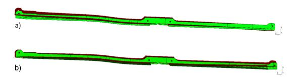
Figure 5-17: Side views of the CAD model for part B (in green) compared with scan data in a free-state (in brown) with a) bending deformation b) torsion deformation.
