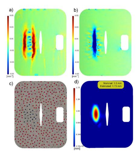
Figure 4-21: Part A with a big (global) defect and bending a) distribution of the difference in maximum curvature  $(K_1)$  [mm<sup>-1</sup>] b) distribution of the difference in minimum curvature  $(K_1)$  [mm<sup>-1</sup>] c) sample points filtered using the curvature criterion (represented as blue spots) d) comparison between estimated and nominal size of defects [mm] when using GNIF sample points after filtering based on the curvature criterion.
