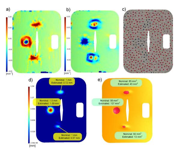
Figure 4-9: a) distribution of the difference in maximum curvature  $(K_1)$  [mm<sup>-1</sup>] b) distribution of the difference in minimum curvature  $(K_2)$  [mm<sup>-1</sup>] c) sample points filtered using the curvature criterion (represented as blue spots) d) comparison between estimated and nominal size of defects [mm] when using sample points after filtering based on the curvature criterion e) estimating the area of defects [mm<sup>2</sup>].
