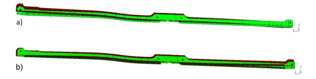
Figure 4-28: Side view of CAD model for part B (in green) compared with the scanned model (in brown) a) with bending deformation b) with torsion deformation.
