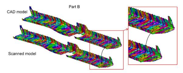
Figure 4-27: GNIF corresponding sample points (in black) on the CAD and scanned models of part B.
