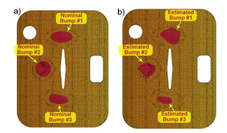
Figure 5-8: defects are identified as red zones based on the tolerance value (0.4 mm) a) for nominal defects b) for estimated defects.
