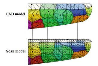
Figure 2-10: Corresponding sample points (black points) generated on the CAD and scan models for a turbine blade (Radvar-Esfahlan and Tahan 2014).
