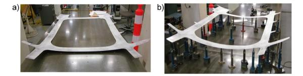
Figure 5-1: A regular aerospace panel, a) in free-state, b) constrained by fixing jigs on the inspection fixture [2].
