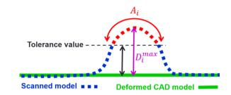
Figure 5-5: Definition of maximum amplitude  $D_i^{max}$  and area of a defect  $A_i$ .
