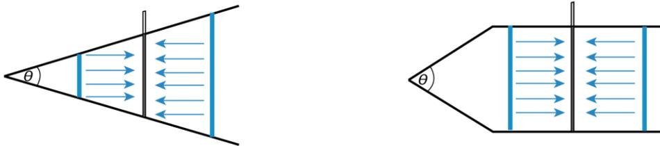
**Figure 2.13. Conceptual flow model of a confined aquifer with a well located a) close to; and b) further away - from a pinch-out boundary (modified from Horne and Temeng (1982) and Mijinyawa and Gringarten (2008)).**
