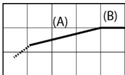
Aquifer cross-cut by a strongly inclined finite-conductivity fault <sup>(6, 35)</sup>. Leaky fault  $n = 1.5$  (bilinear) flow (A). Late radial flow (B) occurs after the matrix signature has masked the
