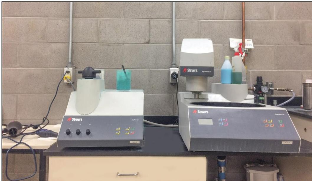
Figure 3.10: (L) Struers LaboPress-3 and (R) TegraForce-5 machines, for mounting and polishing samples for metallography.
