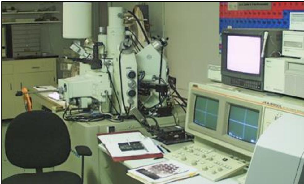
Figure 3.9 : JEOL JXA 8900L WD/ED electron probe microanalyzer coupled with a wavelength dispersive spectrometer (WDS).
