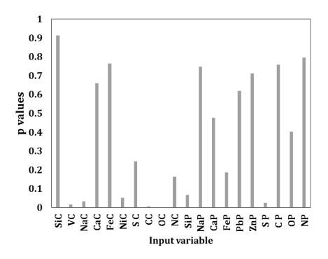
**Figure 5** 'p' value for different input (chemical compositions and impurity contents of coke and pitch) variables (XC denotes element X in coke, XP denotes element X in pitch)
