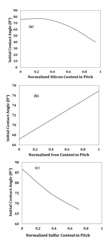
Figure 4 Effect normalized pitch impurities on contact angle at 80 s (a) silicon (b) iron (c) sulfur
