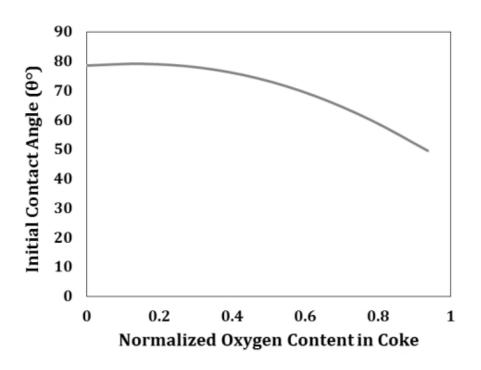
**Figure 3** Effect normalized oxygen content in coke on contact angle at 80 s
