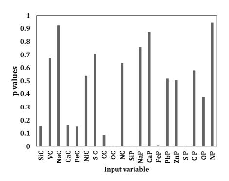
**Figure 1** "p" value for different input variables (chemical compositions and impurity contents of coke and pitch) for contact angle at 80 s
