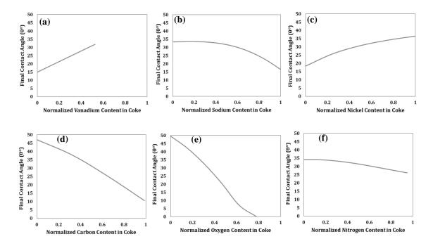
**Figure 7** Effect of normalized coke chemical compositions and impurities on contact angle at 1500 s (a) vanadium (b) sodium (c) nickel (d) carbon (e) oxygen (f) nitrogen
