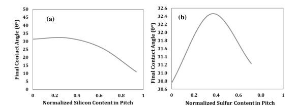
**Figure 8** Effect normalized pitch impurities on contact angles at 1500 s (a) silicon (b) sulfur
