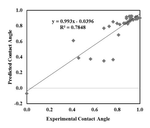
Figure 2 Normalized predicted vs. experimental contact angles at 80 s
