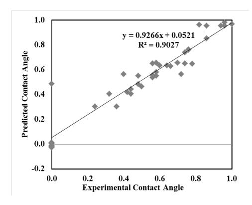
Figure 6 Normalized predicted vs. experimental contact angles at 1500 s
