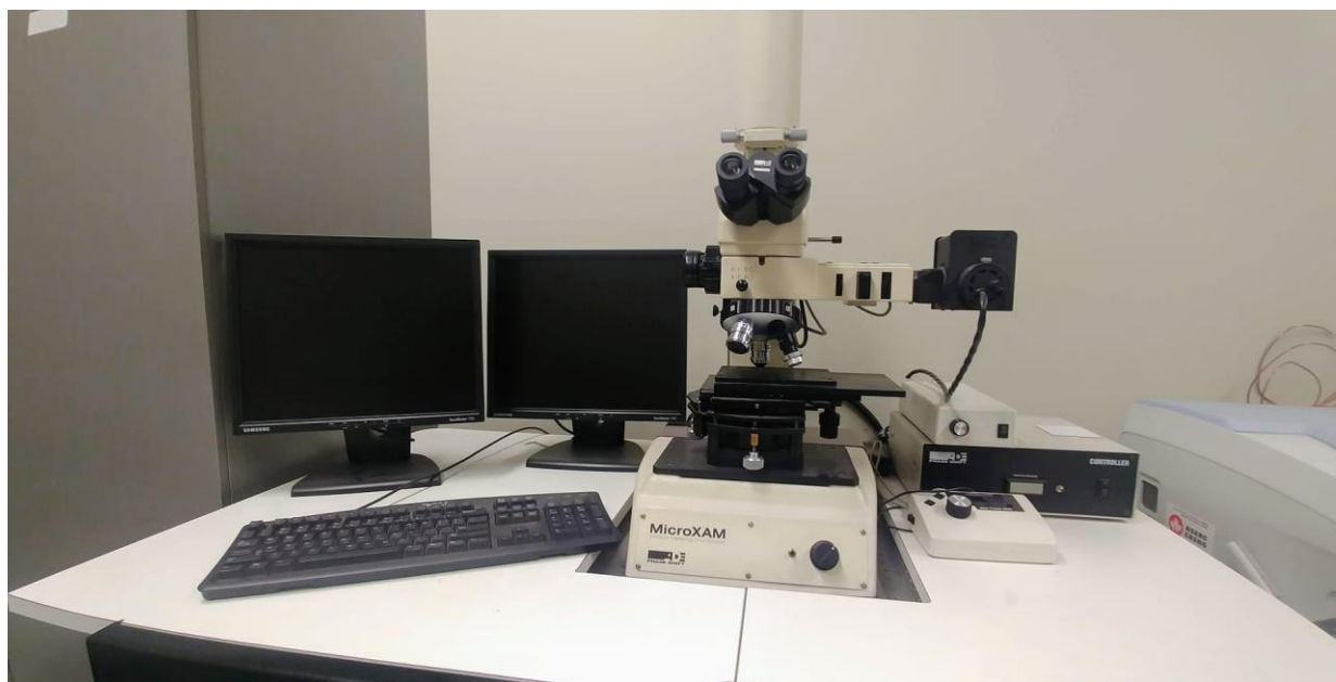
Figure 3.4: Instrument of Optical profilometry
