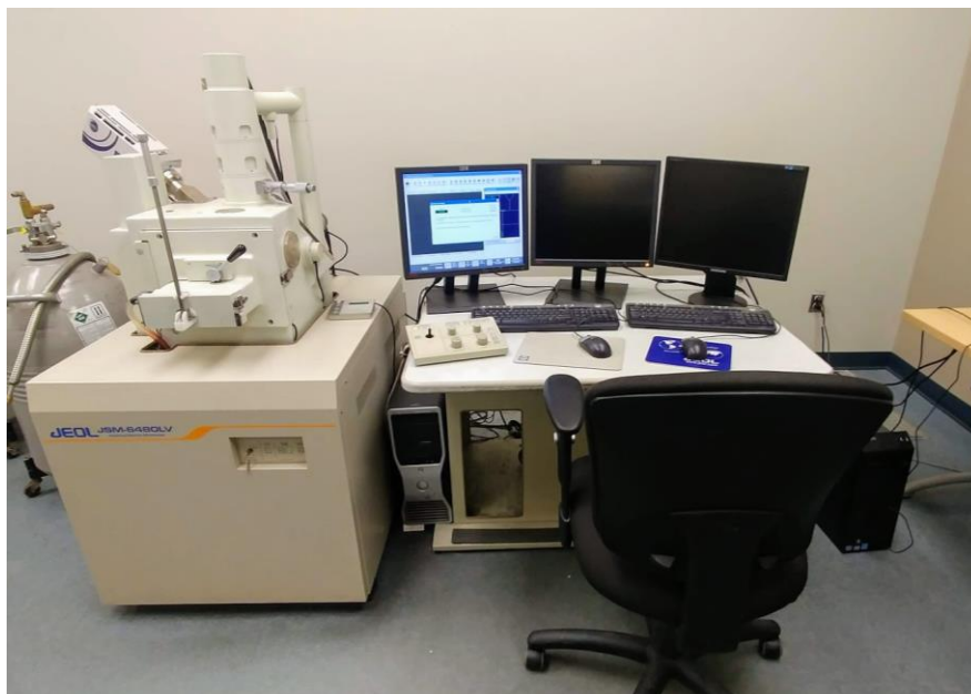
Figure 3.3: Scanning Electron Microscope SEM Jeol (model JSM 6480LV) instrument.
