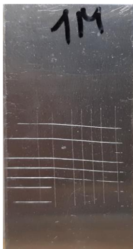
Figure 4.9: Adhesion test on Al substrate coated with sodium silicate thin film formed using 1 M sodium silicate solution.
