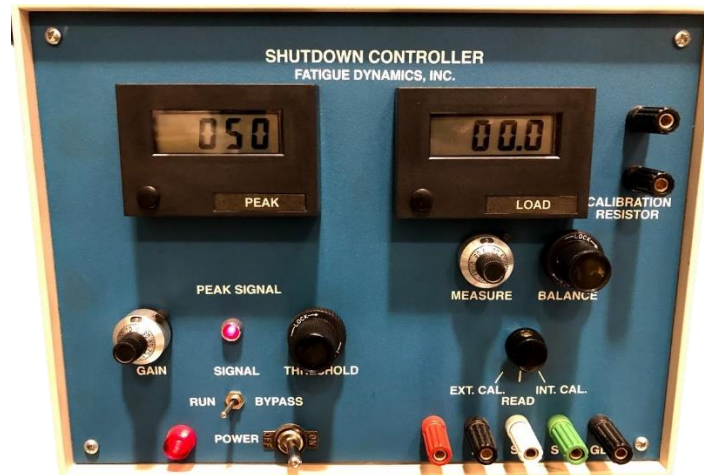
Figure 3.31: Shutdown controller of bending fatigue machine.
