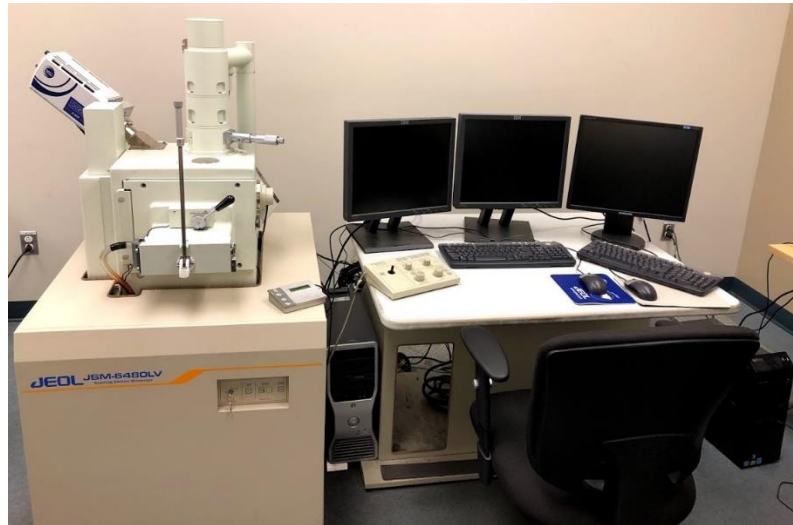
Figure 3.22: Scanning electron microscope used in examining the fracture surface of failed control arms.
