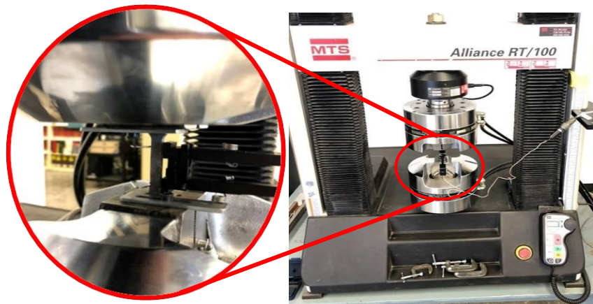
Figure 3.12: Set up of tensile test.
