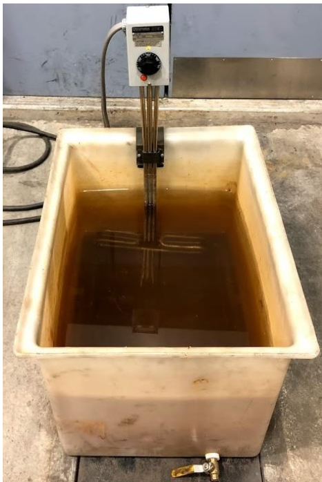
Figure 3.3: Quenching medium maintained at 60 °C by means of electric heater.
