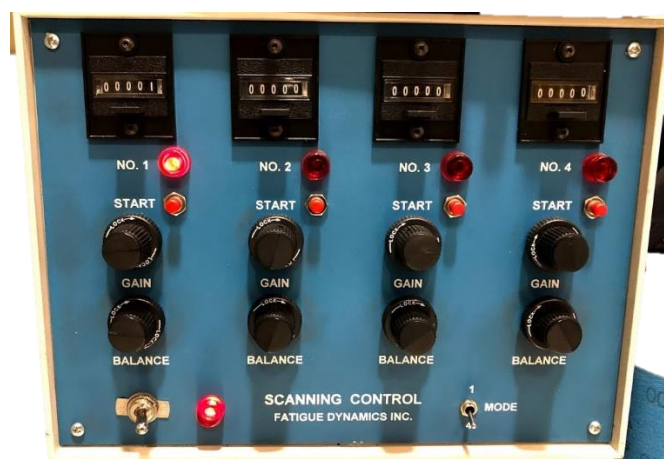
Figure 3.32: Scanning controller of bending fatigue machine.
