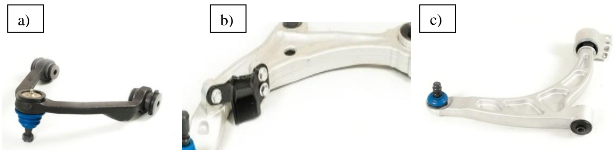
Figure 1.5: Different designs of control arm a) Press-In, b) Bolt-In and c) Unitized [16]. Complete understanding of the importance and functions of different types of suspension systems helps in applying the proper loads to the suspension arm in this study. Suspension control arm of interest in this study is explained in the next subsection.
