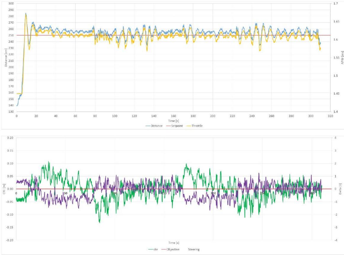
Figure 6: Results from the walking experiment a) Distance control primary axis and throttle output on the secondary axis; b) Perceived cross track error (primary axis) presented with the steering response (secondary axis).
