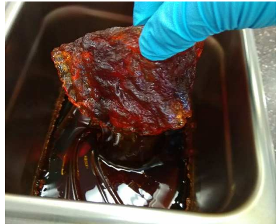
Fig. 1. Gelling of natural ester under open beaker aging conditions in laboratory.
