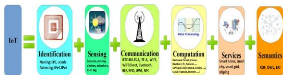
Figure V-1 Six main elements needed to provide IoT functionality. © 2021 Ghassan Fadlallah & IEEE Com.
