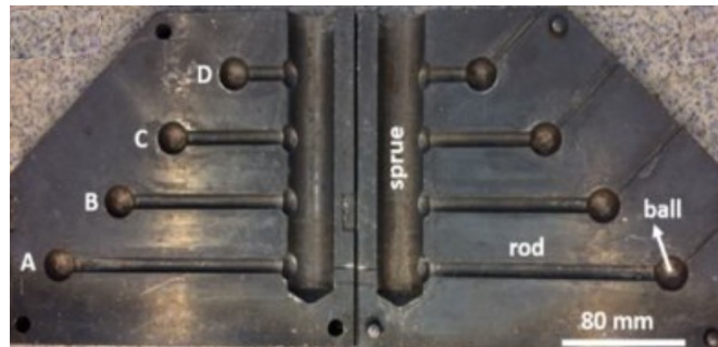
Figure 2-7. Mold for constrained rod casting (open access) [55]
