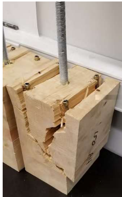
Figure 3: Failure by splitting through the screws.
