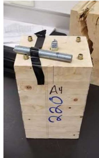
Figure 15: Yielding of the steel rod (failure type B)
