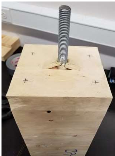
Figure 14: Wood shearing around the rod (failure type A)
