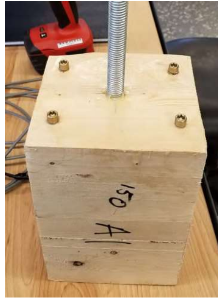
Figure 2: « Pull-Pile foundation » specimen
