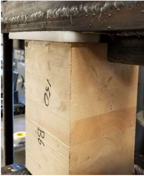
Figure 4: Teflon layer for « pull-push » tests.
