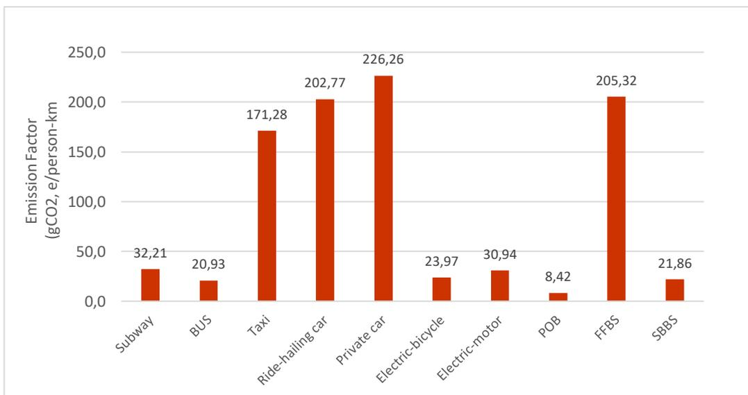
Fig. 8 Greenhouse gas emission factors for various modes of transportation in Beijing, the GHG emission factor of the bus is calculated based on the weighted average of the number of two different types of buses.
