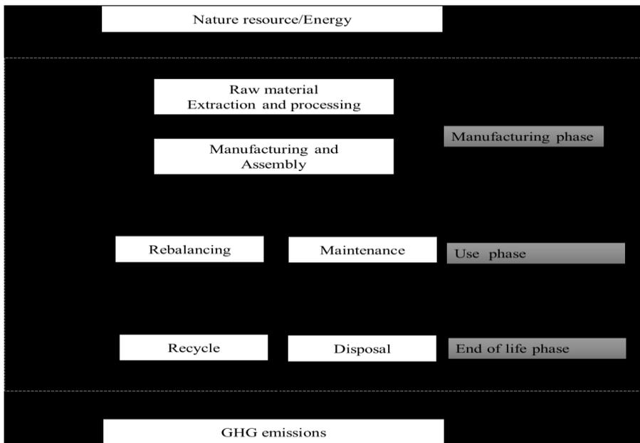
Fig. 5 The LCA frameworks for non-energy-powered vehicles
