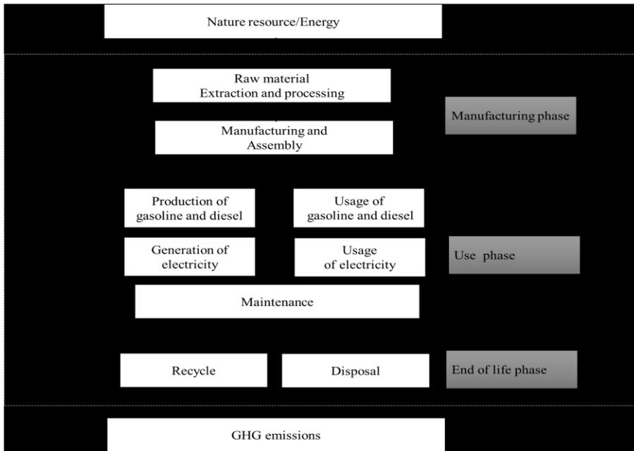
Fig. 4 The LCA frameworks for energy-powered vehicles
