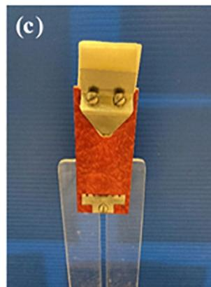
**Figure 3.** (a) Schematic illustrating the test setup for inclined plane test (IPT); (b) and (c) parts used for mounting the samples for IPT.
