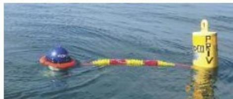
Equipped with an external battery pack, the HydroBall® buoy can be moored up to 30 days for water level and wave measurements campaigns.
