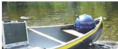
Dropped upstream, the HydroBall® buoy autonomously collects bathymetric data while drifting.
