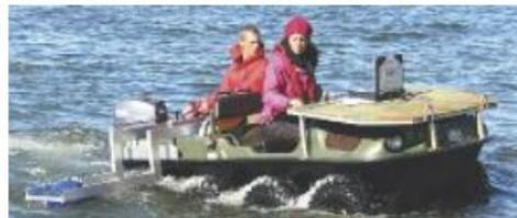
Mounted on an amphibious vehicle, the HydroBall™ buoy can produce continuous land-sea profiles for integration of continuous land and sea data.
