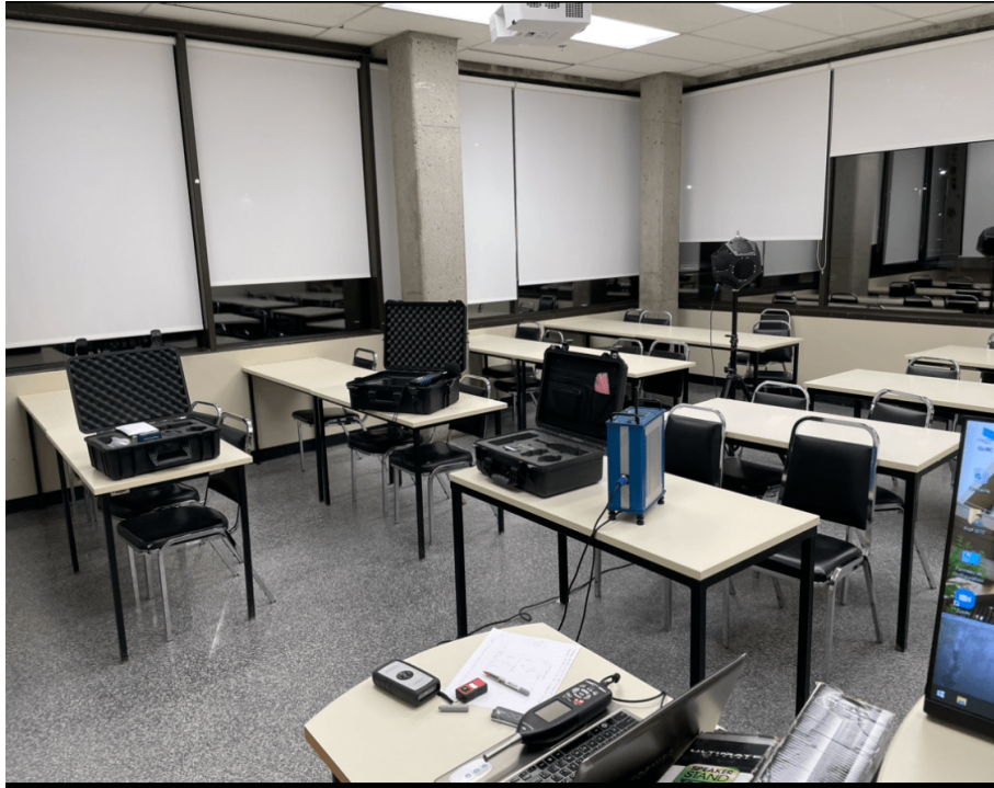
Figure 4.12: Acoustic measurements set up in a classroom at University of Quebec in Chicoutimi.
