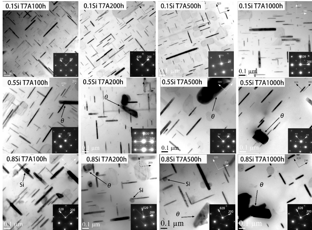
Figure 4.5 BF-TEM images and corresponding SAEDPs of experimental alloys at different T7A conditions.
